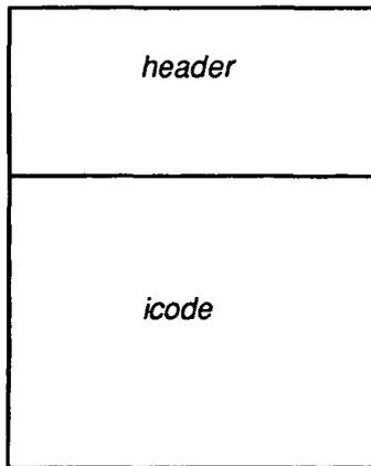
The icode part contains the operations and data specifications that make up an Icon program. The header is the part that allows the icode file to be directly executable as a command, without having to type `iconx`.
