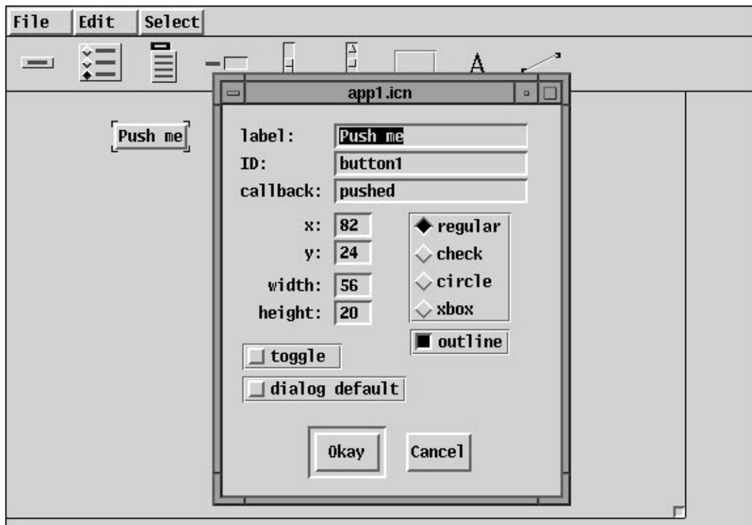
If the Okay button is selected VIB checks to ensure that entered values are valid. For example, if there is no value entered into the x-coordinate field, an error dialog appears describing this error. The error dialog disappears when either the Okay button is selected or the return key is typed. This in turn redisplay the attribute sheet until the error is corrected or the Cancel button is selected.
