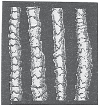
SERRATIONS, as seen on Wool Fibre.
