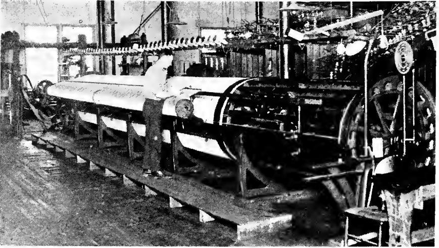
THIS picture shows the huge beam onto which the thread is finally wound before it is put into the machine. It forms a body, constituting the warp of the fabric.
