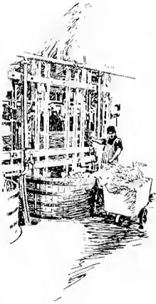
The washing process, in another tub, is also carried on on the same principle—pounding of electrically-operated wooden mallets on the fabric to loosen the dirt. It is then bleached with solutions of lime and acid. After rewashing, the goods go into the centrifugal wringer where swiftly-revolving circular plates making 3,000 revolutions per minute whirl it against the smooth, curved sides, wringing the water out without injury to the lace.
