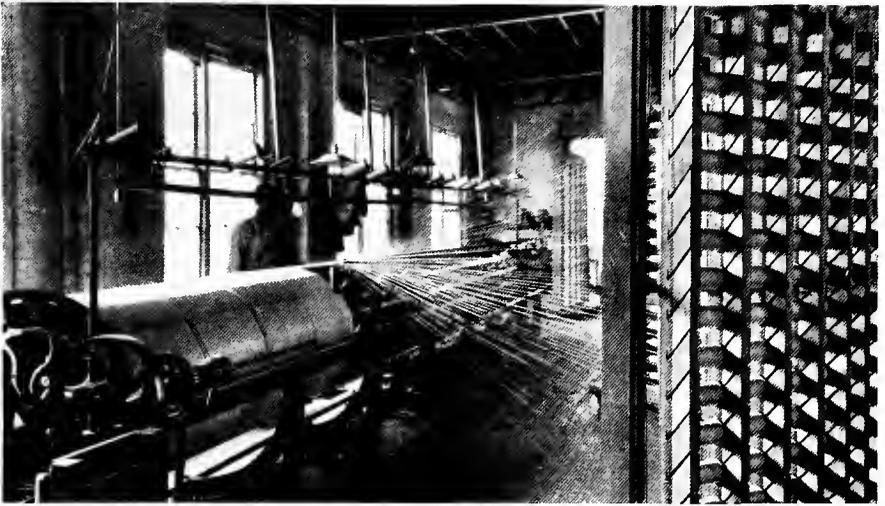
AFTER inspection the skeins of yarn are placed on revolving racks to be wound by machinery onto spools. One machine can wind 300,000 yards a day, the operator's sole duty being to watch for broken threads and to tie them. Her fingers must be nimble and her eyes alert to detect a break in the scores of flying lines of fine thread.
