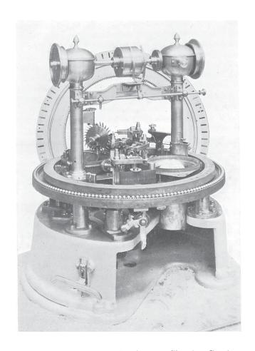
Fig. 96.—The Noble Horizontal Circular Comb
