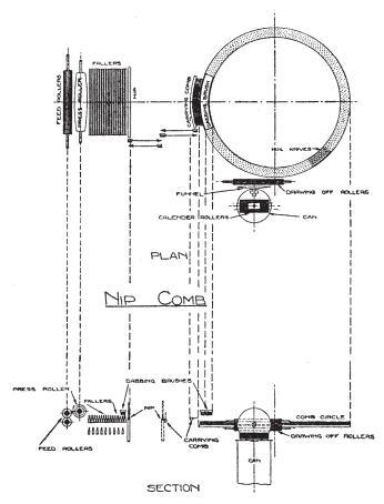
Fig. 100.—Plan and Section of Nip Comb
