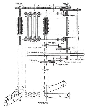
Fig. 87.—Plan and Section of "Sheeter" Preparing Box
