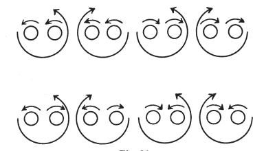
$\begin{array}{c} \text{Fig. 86}_{\text{B}} \\ \text{Illustrating the various conditions of twisting a simple} \\ \text{two-fold yarn} \end{array}$
