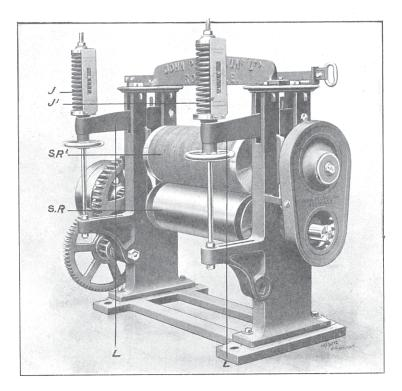
Fig. 21. Arrangement of Squeezing Rollers as applied to Petrie's Wool Scourer.
