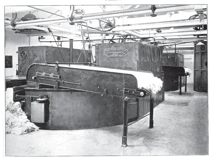
Fig. 29a. Installation of Stone's Dryer.
