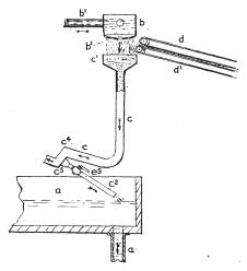
Fig. 24. Section of Conduit Machine showing Feed Arrangement.
