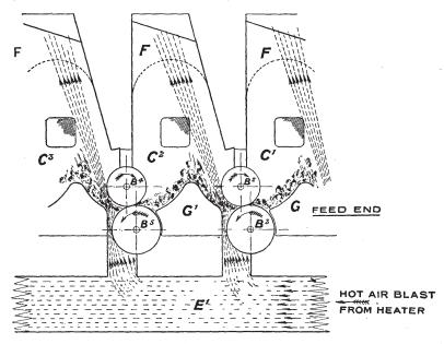
Fig. 26a. McNaught's Continuous Wool Drying Machine (Compartment Method), showing direction of currents of heated air and their action on the wool.
