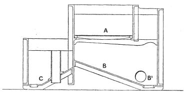
Fig. 17. Vertical Cross Section of McNaught's Wool Scouring Machine.
