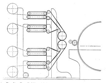
Fig. 74. Four-Bobbin (with four pairs of rubbers) Tape Condenser.
