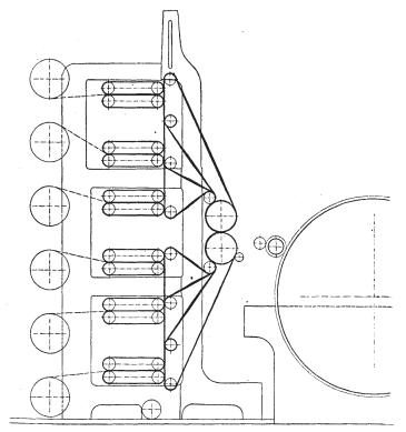
Fig. 75. Six-Bobbin (with six pairs of rubbers) Tape Condenser.
