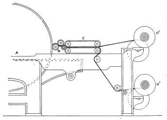
Fig. 70. Single-Rubber Condenser.
