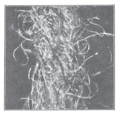
Fig. 81. Condensed Sliver after Drafting, Pulled Waste.
