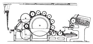
Fig. 67. Over first small Cylinder, A, Burr-Roller is fixed, and over the second Cylinder, A, a Worker and Stripper.
