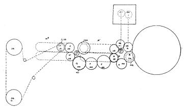
Fig. 71. Driving Mechanism for Single Stripper Tandem Condenser.
