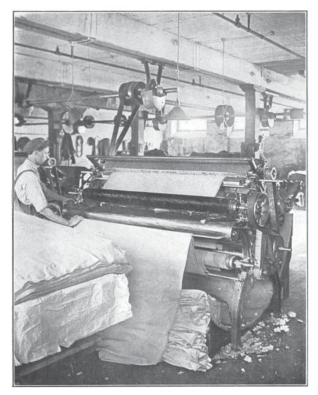
CLOSE-UP OF A SHEARING MACHINE IN A GREAT WOOLEN ESTABLISHMENT. NOTE THE PILES OF CLOTH WHERE IT HAS LEFT THE MACHINE
