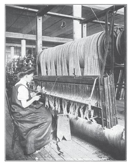
DRAWING WARP THREADS THROUGH THE HEDDLES IN THE HARNESSES, WHICH CONTROL THE APPEARANCE OF THE WEAVE, AS THEY MOVE UP AND DOWN AC-CORDING TO THE PATTERN
