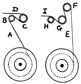
Fig. 28. Extra Back Rails for Warp Tension.
