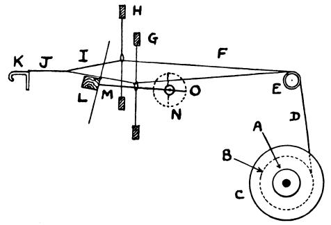
Fig. 27. Outline of Warp from Warp Beam to Breast Beam.
