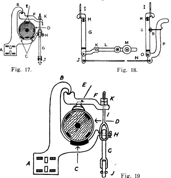
Fig. 17. Briggs's Let-off Motion (End View). Fig. 18. Front View. Fig. 19. End View with only One Bottom Cap.
