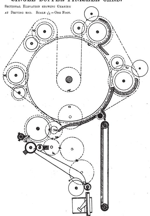
Sectional elevation showing gearing at opposite end to driving pulleys.
