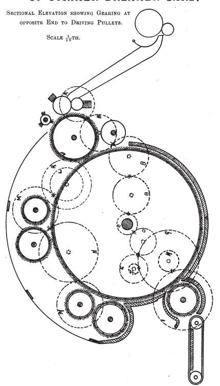
Sectional elevation showing gearing at end opposite to driving pulleys.
