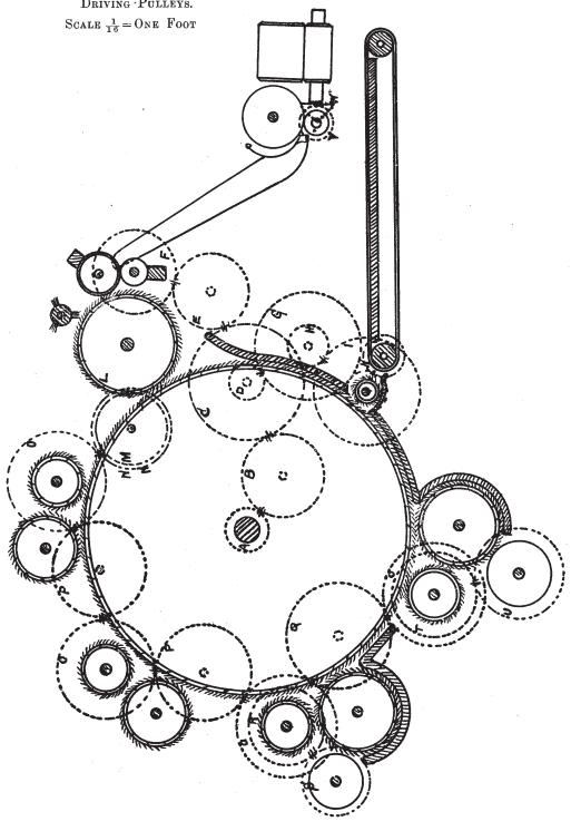
Sectional elevation, showing gearing at driving end.
