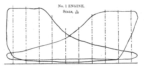
Mean Pressure—Front, 33 7 lbs. Mean Pressure—Back, 31 7 lbs, Average Mean Pressure—32 7 lbs. per sq. inch.
