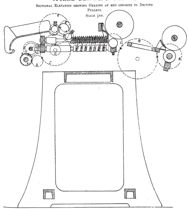
Sectional elevation showing gearing at driving end.
