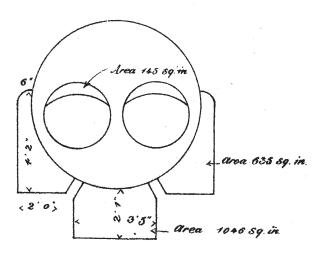
The centre flue is about three feet wide and two feet deep, and the side flues about two feet wide at the bottom, and at the closing-in (which is about three-fourths of a circle) about nine inches wide.
