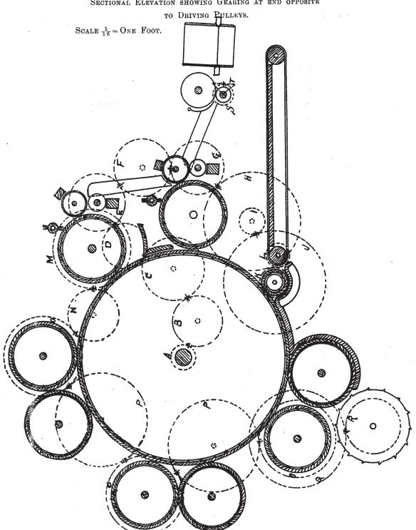
Sectional elevation showing gearing at driving end.
