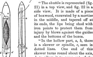
side view. It is made of a piece of boxwood, excavated by a mortise in the middle, and tapered off at its ends, the lips being shod with iron points to protect them from injury by blows against the guides and the bottoms of the boxes. "In the hollow part, a, b, there is a skewer or spindle, c, seen in
