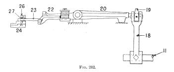
groove for the action of the bent depressor rod 23. The free end of rod 23 rests upon the top side of the feeler bracket 24, and, so long as there is sufficient weft in the shuttle, it is kept by spring action hard against the front of the bracket. Under these conditions, the feeler lever
