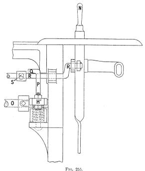
will clearly place the short arm S under the bent portion Q of the rod P. If the shuttle does not reach the box, the tongue F will come into contact with the front of the frog H, and the latter will, in moving slightly round O, cause the end H<sup>1</sup> to pull down rod P, and so cause the cranked end of rod R, Fig. 255, to pull the handle N out of its
