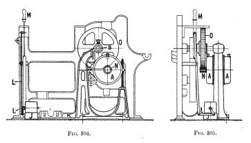
enough to drive the loom when all is working properly, and the grip of the brake may be strengthened or weakened at will according to requirements. Apart from the pinion, wheel and brake, the arrangement is very similar to that illustrated in Figs. 302 and 303, and the essential parts are again shown up in heavy lines.
