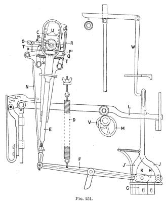
loom. Opposite ends of bracket G also serve as supports and fulcra for the ends of the short lever H which couples the lower ends of the vertical draw hooks J J<sup>1</sup>, and also compounds the latter with lever F by means of pin or stud K.
