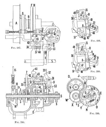
pin Q enters one of the recesses R, the main shaft S of the automatic motion commences to rotate. Fixed securely on this shaft, and working in perfect unison with each other, are five tappets, 1, 2, 3, 4, and 5, for operating the different
