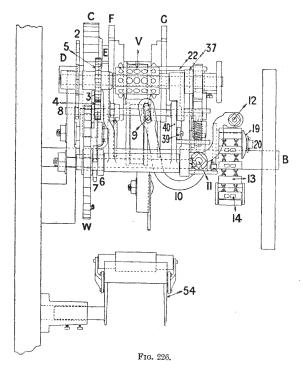
plates prevent all motion on the part of the eccentrics except when the teeth of R and S come into contact with the teeth on discs F and G.
