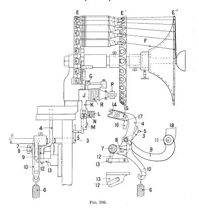
Transfer hammer G is returned to its position of inaction by a coiled spring R, Fig. 280, and, as the hammer returns, the hopper E is partially rotated clock-wise by the following means to bring the next pirn under the hammer head.
