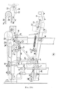
V is the ordinary set-on handle of the loom, and controls, as shown, the electrical switches in box W—the loom being driven by a small motor. A second handle X is provided for the purpose of controlling certain mechanism when the plain part, border or otherwise, is to be woven. When it
