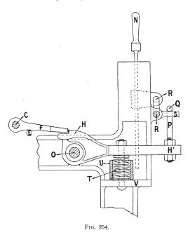
tongues F which are lifted when the shuttle is in the box by rod E which forms the lower cranked part of the finger. The action is almost identical with that explained in connection with Figs. 252 and 253 when the loom is running, i.e. the tongues F clear the knees or frogs H. In Figs. 254 and 255, however, the frog does not slide, but is capable of being slightly rotated upon the rod O. The
