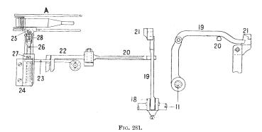
the arm 20 of the feeler lever and enters a slot in the specially formed head 21 of the weft fork hammer. Arm 22 of the feeler lever is forked at the end to provide a cam
