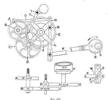
sliding block Y. The values of the wheels are different from those given in Fig. 212, but the number of teeth in each wheel is indicated in the distorted plan view of the motion in the lower part of the figure. Theoretically, the practice of connecting rod K with the wyper shaft is objectionable, as the cloth is taken forward only every second pick, but the arrangement is extensively used, and is
