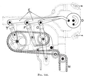
positions; but, since there are three more bushes (marked 2 on the chain) to appear in successive order under lever C, it follows that no movement will be given to wheel D, hence the box remains stationary for four picks. The lever Y is for the picking arrangement (see Fig. 186, and explanation on p. 351).
