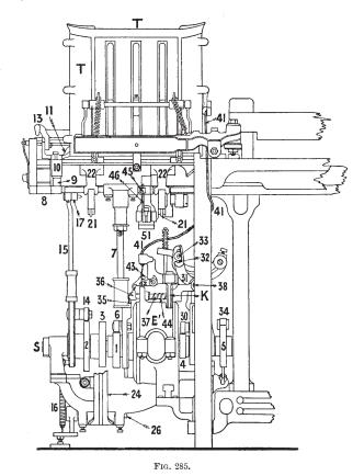
the outward movement of pin M is due to the partial rotation of lever O through the pull of spring N. When the lever O moves as indicated, the clutch pin Q enters one of the recesses R, indeed the first which is presented in virtue
