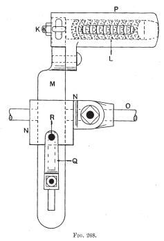
and the temple come in contact. A brass cover P, screwed or snibbed to the holder M, fulfils the double purpose of protecting the weaver and of deflecting the cloth sufficiently to grip the rings L. As these rings rotate with the movement of the cloth, the first point of contact of the latter with the rings compels the cloth to move outwards, this
