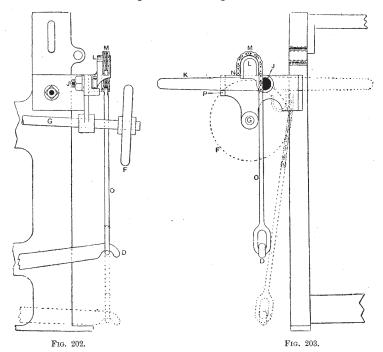
hold the lever K more firmly in its normal or proper position (i.e., resting upon the projecting part P of the bracket) and make it impossible for any accidental relief to be given to the beam. This fact constitutes the great advantage of this method of arranging the relieving bracket over that of the common quadrant type, which,
