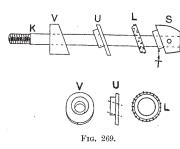
washer is slightly longer than the thickness of the rings L in order that the latter shall have freedom to rotate. The clearance, however, is small, and in order to obtain the best results the temple must be kept scrupulously clean.
