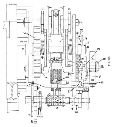
quently, makes one revolution for two picks. Projecting from the two faces of wheel W are pins Y and Z; the latter drives cylinder V clockwise directly by means of wheel 2, while the former drives the cylinder counter-clockwise by
