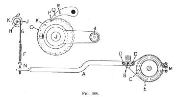
breast beam. The larger detached figure shows that at the ratchet wheel end of shaft J a handle L is provided, by means of which the shaft may be partially rotated, thereby lowering lever A, and removing the pressure from the drag head. Naturally any downward movement of the long arm of the lever A will cause both pins D to slacken band E, since the two pins are on opposite sides of the fulcrum B.
