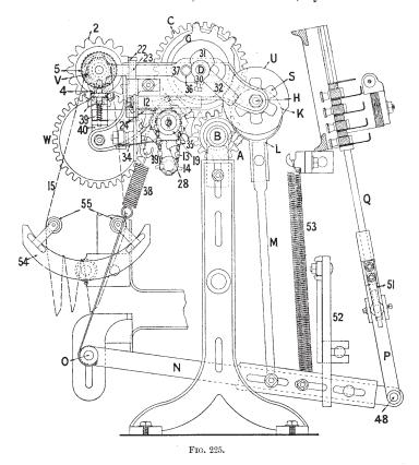
rod M, whilst the outer end of lever N is connected to the boxes by means of part P through the safety escapement mechanism and plunger rod Q. The double eccentric K is similar to that illustrated in Fig. 230.
