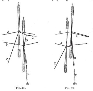
under the crankshaft as indicated, instead of over the lease rods, any tendency to increase the strain upon that thread when forming the crossed shed is greatly minimised. In weaving these selvages the proper pacing of the bobbin from which the thread C is drawn is a most important feature; indeed, the production of a perfect selvage, as well as the ensuring of a minimum of trouble to the weaver, depends almost entirely on this adjustment.
