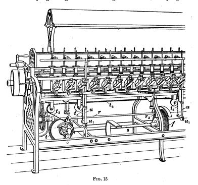
segment  $t_2$ . Connected to the segment is the chain  $t_3$  that operates the rod  $t_4$  and chains  $t_5$ , the chains  $t_5$  being connected to the lifting-rod dogs  $u_1$  attached to the lifting rods u. Since the mangle gear is driven first in one direction and then in the other by the pinion gear, the gear t will also reverse its direction of motion at regular intervals. This will impart a swinging motion to the segment arm  $t_1$  and
