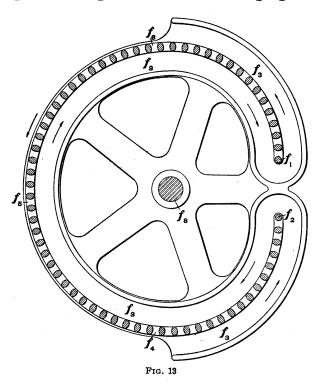
13. Reference is now made to Fig. 13, which shows the mangle gear alone in cross-section. This gear is composed of two rings joined together by pins that form teeth. By this means, the pinion gear engaging with the mangle wheel can drive it either from the outside or the inside of the teeth. It will be noticed that the teeth of the mangle gear end at the points  $f_1$  and  $f_2$ . This is to allow the pinion gear engaging
