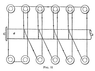
they will revolve in the direction opposite to that of the hands of a watch, thus causing the ends when being wound to pass to the right-hand side of the spool.
