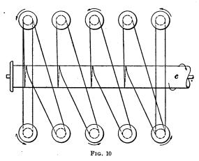
double whorl, and consequently two bands. This method of banding is clearly shown in Fig. 10, where five spindles on each side of the frame are shown; c shows the cylinder of the spooler, around which the bands pass and thus receive their power. In some cases when spindles are banded in the manner just described, instead of providing spindles with a double whorl, the last band at each end of the frame will drive three spindles instead of two.
