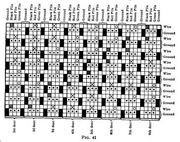
pile in Fig. 41. For instance, suppose that the shaded squares in Fig. 40 represent black, the crosses red, and the circles green. On the first pick of Fig. 40 there are 2 black, 3 red, and 3 green. By referring to Fig. 41 it will be seen that this is exactly the manner in which the pile is formed over the first wire. The pile is lifted over the second wire according to the second pick of Fig. 40, and so on.
