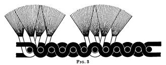
pile will have a tendency to remain in the center of the cord, while the shorter pile will be on each side, thus giving the desired rounded appearance of the cord when finished. Fig. 3 shows the appearance of the section in Fig. 2 after the pile filling has been cut.
