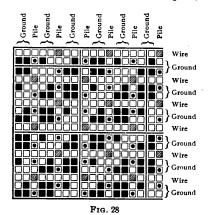
what is known as *Utvecht velvet* is shown; when the first wire is inserted every alternate end of the pile warp is raised over it, and when the next wire is inserted those ends
