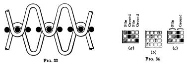
in Fig. 34 (b), while in view (c) the corresponding chain draft is shown. It should be noted that the ground ends in Fig. 34 (a) are interlaced with the picks situated between the upper and lower pile loops to prevent the filling from
