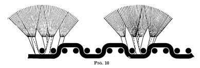
the ground cloth by being passed under only 1 end of the warp, but in some varieties of filling-pile weaves the pile picks are bound more securely by being passed under one end, over the next, and under the third, before floating, which causes the weave to require a larger number of ends in the repeat in order to obtain any given length of pile-filling float.
