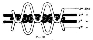
being forced out with the loops of pile warp. This will be more clearly understood by referring to the section in Fig. 35, which illustrates not only the interlacings of the pile ends in Fig. 34 (a), but also of the ground ends.
