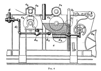
it is to be used for rayon sizes. Some of the old-type size boxes that are still in use have a cast-iron frame that supports a wooden size box. In some instances, the wooden box is lined with a suitable material, while in other cases, the size is held in the unlined wooden box.
