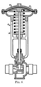
overcome the resistance of the spring and close the valve. But, as the air pressure in the diaphragm chamber is reduced, the spring will gradually open the valve. Not all diaphragm motor valves are constructed to act in this manner. Some valves are built to be opened when air pressure is applied and closed when it is reduced.
