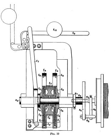
permit a slight lateral movement. These sleeves, however, are not free to revolve without turning the shaft to which they are keyed. Attached to these sleeves are two friction plates  $t_1$ , which consist of thin steel disks covered on both sides with friction pads  $t_2$  of a material possessing a high coefficient of friction,
