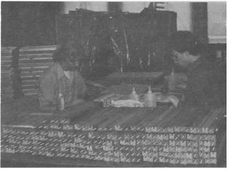
Workers gluing dents in warp beams
