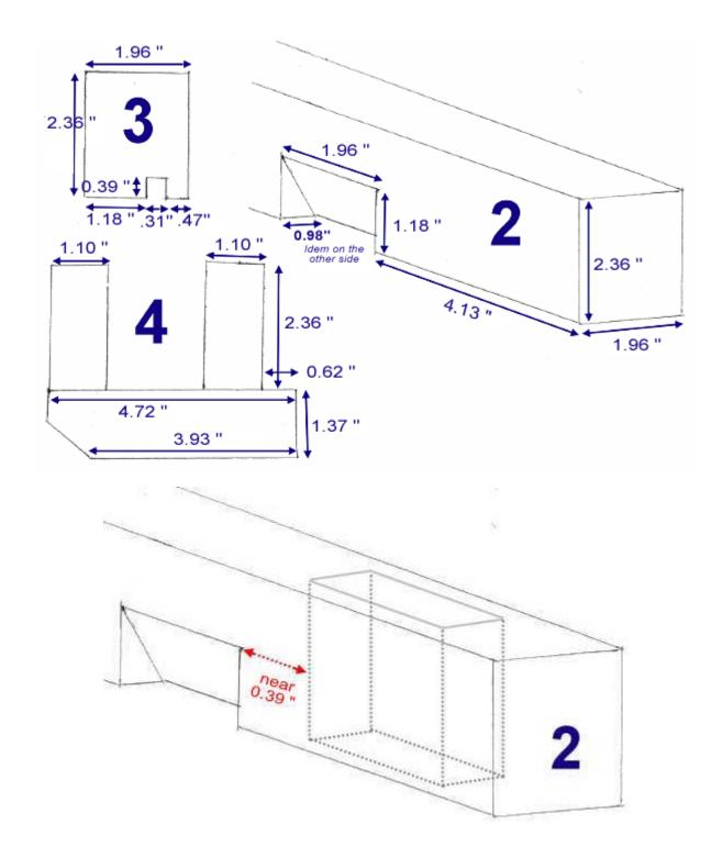
By this hole the arm 1 of the batten passes. The exact dimensions should correspond to the section of arms 1 of the batten, to allow them just to slide inside. The detail 3 possesses the same hole.
