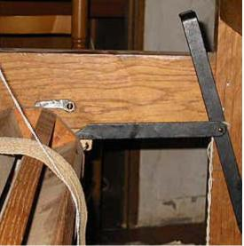
System of blocking of the front roller
