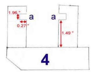
The four small boards of shuttle boxes are grooved on all their length, in a. The groove measures 0.46" deep on 0.19" in height. They should allow to let slide "rats" with a certain space.
