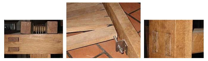
These crossbars can be assembled to the sides of the frame loom by pins and mortises, or joining in middle - wood strengthened by set squares, according to your competence and the material which you have.
