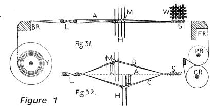
The shed formation mechanism simply divides the warp ends into two groups - one group being lifted while the other is held down - to form an open channel, called the *shed*, between the two warp groups. Once the shed is formed, the weft is inserted through it and then the reed is brought forward to beat up (pack) the newly inserted weft to its desired position. The cycle continued with formation of the next shed...
