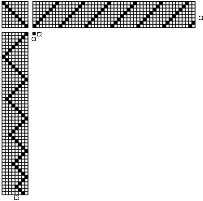
The threading is an upward straight draw. The sequence is:
