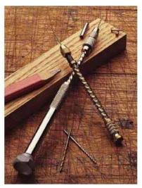
Hand drill or breast drill Watchmakers pump drill Archimedean Drill
