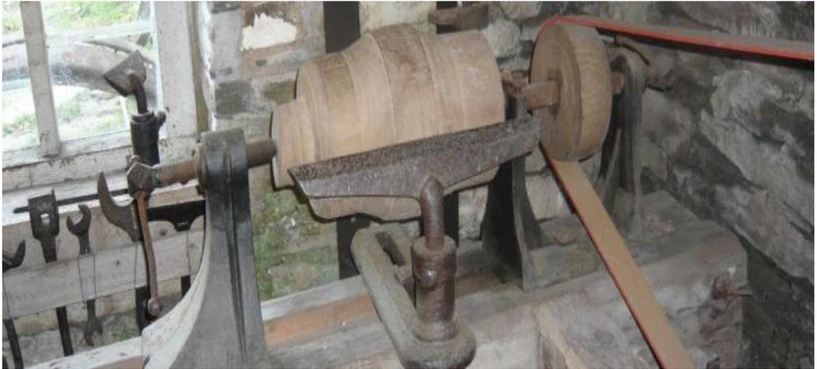
A water-driven lathe
