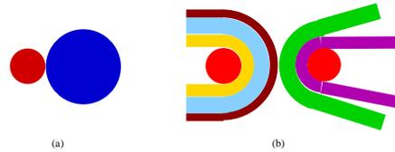
**Figure 3:** The two types of stopping condition: (a) collision of two vertices (b) collision of two elbows.
