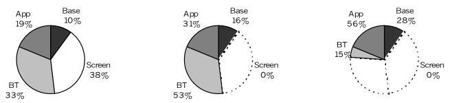
Fig. 2. Power consumption broken down by major components. Left (A) chart shows the power consumption breakdown when all components are active. Center (B) shows the relative power consumption when the screen is shut off. Right (C) chart shows power consumption when the screen is off and Bluetooth power consumption is optimized.
