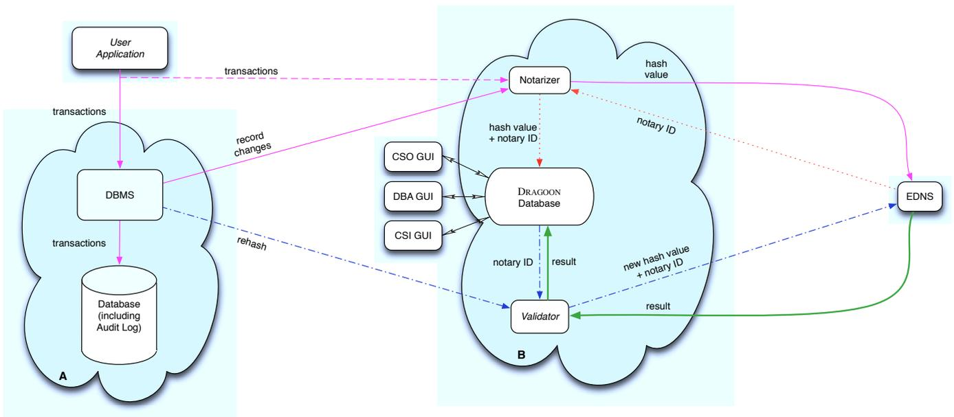
Fig. 2. Normal Processing, Computation of Total Chain, and Tamper Detection of Database in the Cloud.
