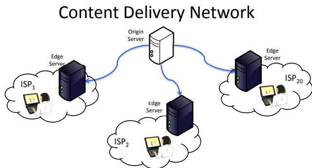
Fig. 1. Content Delivery Network with users being assigned to Edge Servers
