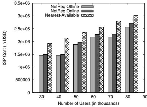
Fig. 6. ISP cost with each server being charged by same ISP charging function (Web Traffic)
