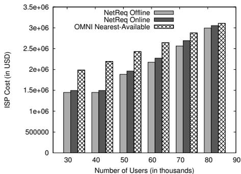
Fig. 3. ISP cost with each server being charged by same ISP charging function (Multicast Traffic)
