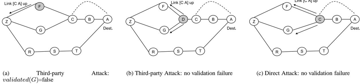
Fig. 7. Third-Party Attack and Direct Attack. The shaded node is an attacker who inject a false link shown in dashed line.
