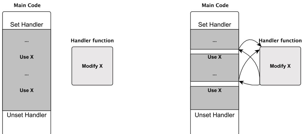
(a) Static CFG of the code. The grey box in the main code appears as a single basic block
