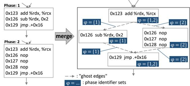
**Figure 4: Merging sub-parts of a basic block. The dashed edges internal to the block are “ghost edges”.**
