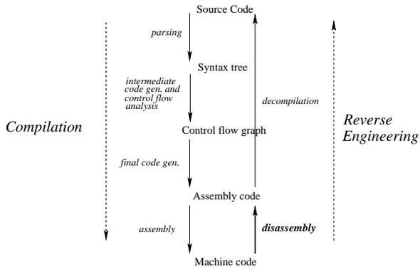
Figure 1: The processes of compilation and reverse engineering
