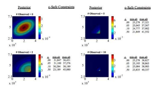
Figure 4: Constraint posterior belief and epsilon-safe constraints after observing 0, 2, 5, and 10 demonstrations from the expert. Axis correspond to the minimum altitude bound (x-axis) and maximum altitude bound (y-axis).
