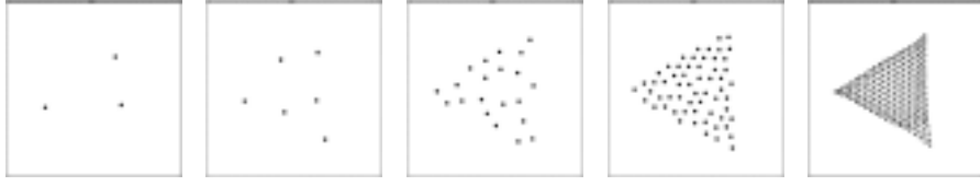
Fig. 2. Drawing of the vertices in the filtration sets. Here \mathcal{V} : V_0 \supset V_1 \supset V_2 \supset V_3 \supset V_4 . The sizes of the sets are 231, 60, 21, 6, 3, respectively. The process begins with a placement for V_4 , followed by V_3 , etc. Note that edges are drawn only when all the vertices are placed.
