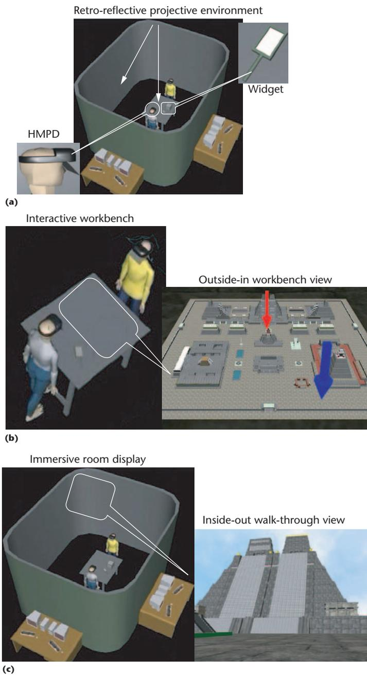
**1 Scap (a) concept and components, (b) simulation of outside-in bench view, and (c) simulation of inside-out walkthrough view.**
