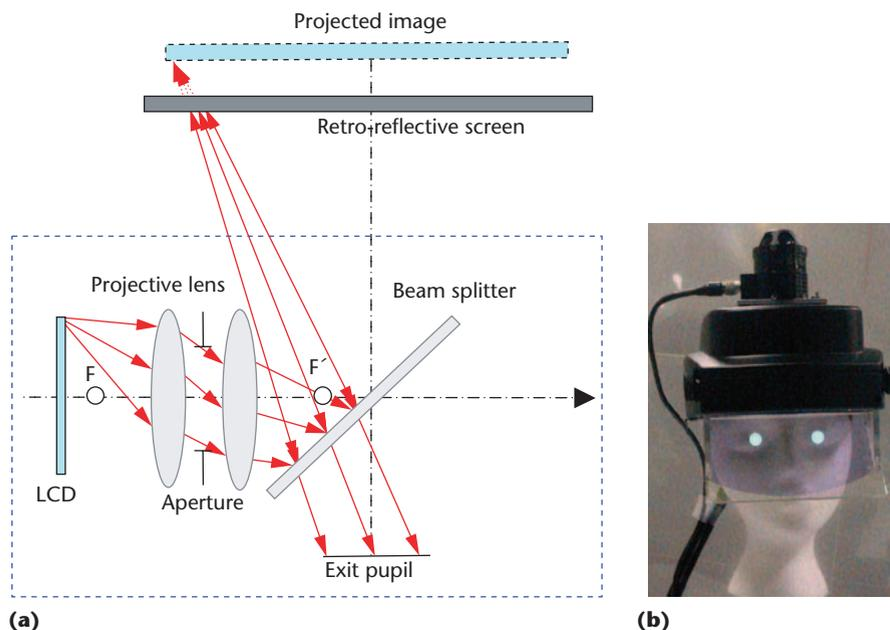
2 Head-mounted projective display: (a) conceptual illustration and (b) compact prototype.
