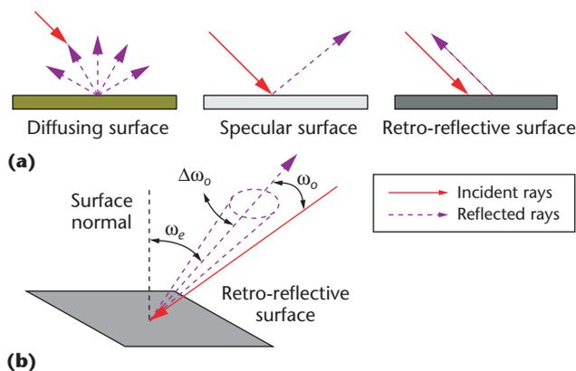
3 (a) Difference in retro-reflection from diffusing and specular reflections, and (b) Characterization of retro-reflective material.
