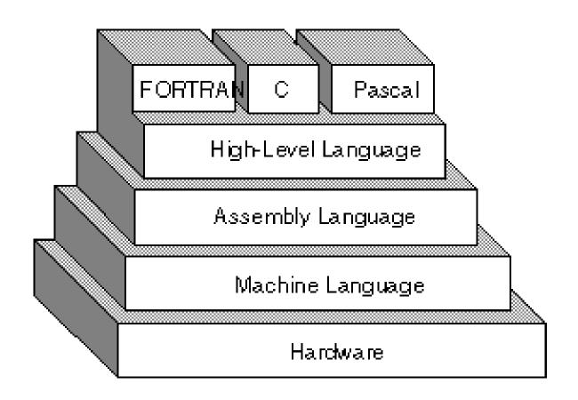
At the "heart" of the computer is the CPU (Central Processing Unit). Each CPU has a language it understands. This language is all in 1's and 0's and is not at all like Python or Java or C, but, if we want to write a program that runs, we have to have a way to create these "machine programs" or executables.
