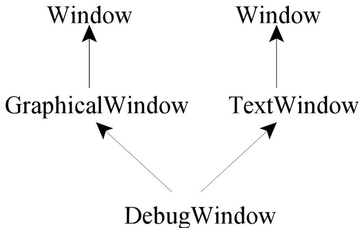
The problem is that both `GraphicalWindow` and `TextWindow` are `Windows`. The constructor for `Window` calls the OS service `CreateWindow()`. Constructing the `GraphicalWindow` portion of `DebugWindow` causes one OS window to be created. A second OS window results from constructing the `TextWindow` portion of `DebugWindow`.
