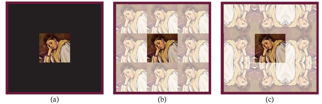
Figure 6.5. (a) Zero padding, (b) circular indexing, and (c) reflected indexing.
