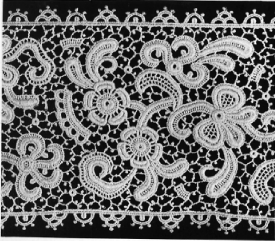
31. IMITATION OF IRISH CROCHET LACE. MADE ON THE SCHIFFLI EMBROIDERY MACHINE. (BURNT-OUT LACE.)
