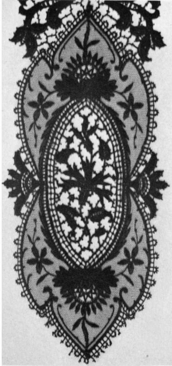
29. BLACK SILK LACE, IMITATION OF MIXED BOBBIN AND NEEDLE-POINT LACES. MADE ON THE SCHIFFLI EMBROIDERY MACHINE.
