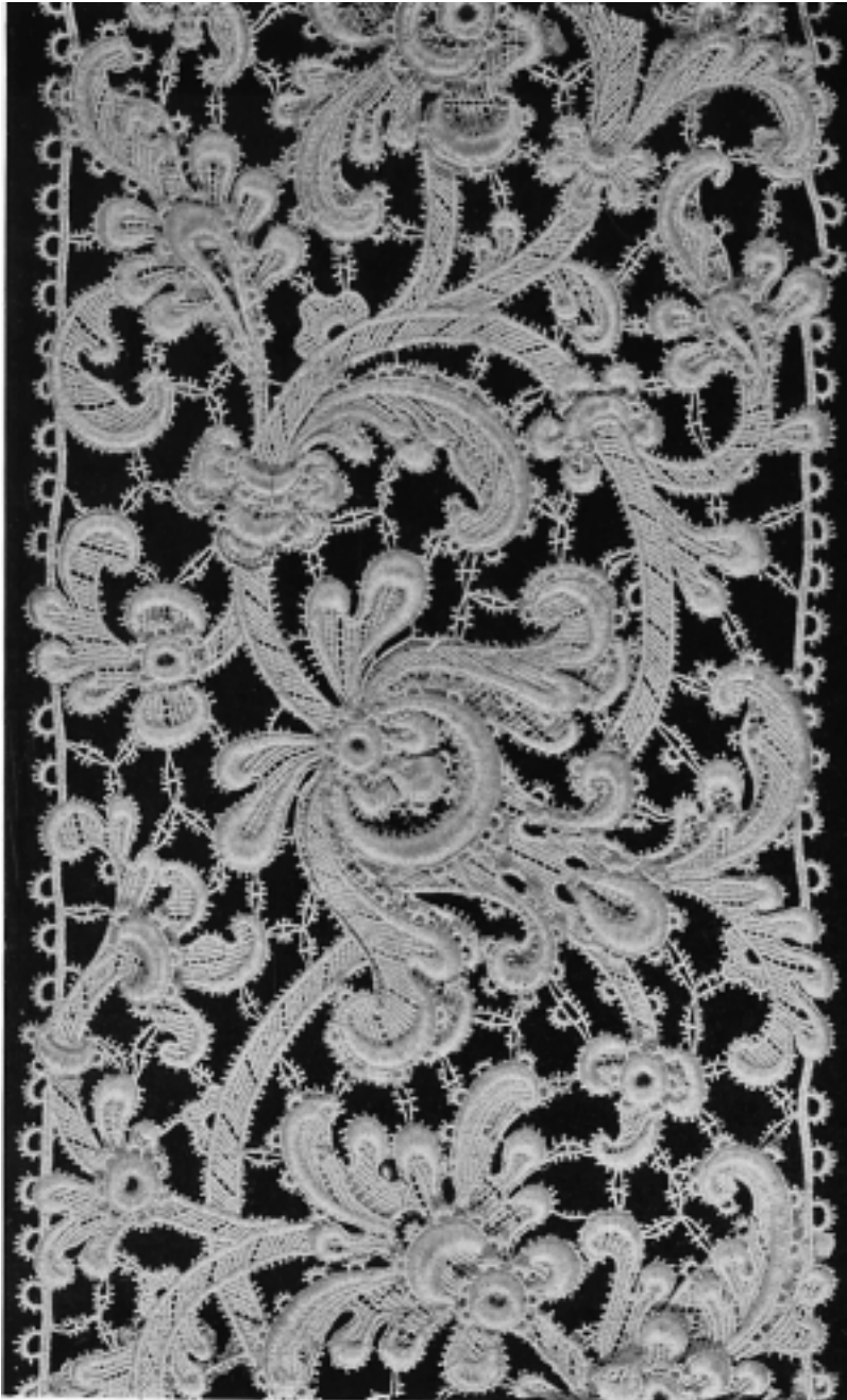
21. GROS POINT DE VENISE, MACHINE-MADE COPY OF HAND-MADE NEEDLE-POINT. MADE ON THE SCHIFFLI EMBROIDERY MACHINE. (BURNT-OUT LACE.)
