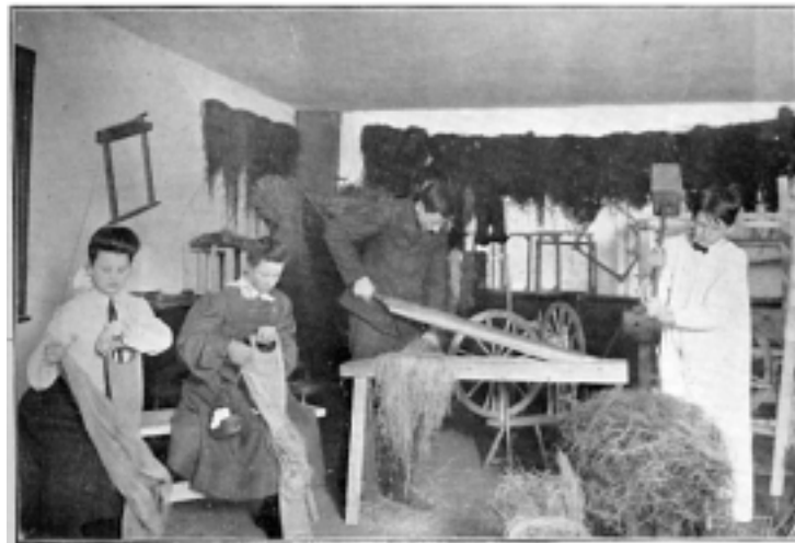
FIG. 2.— Pounding, Breaking, and Hackling.
