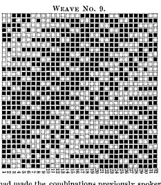
If we had made the combinations previously spoken of from weave No. 4 and 5, and 4 and 6, we could then have produced several others of the 32-harness variety, but they would all run into that sameness with a difference in positions; therefore, weave No. 9 is the only independent combination that can be produced from the above on the principal followed.
