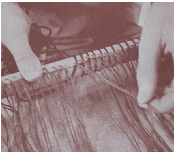
Detail of securing warp to dowel rods.
