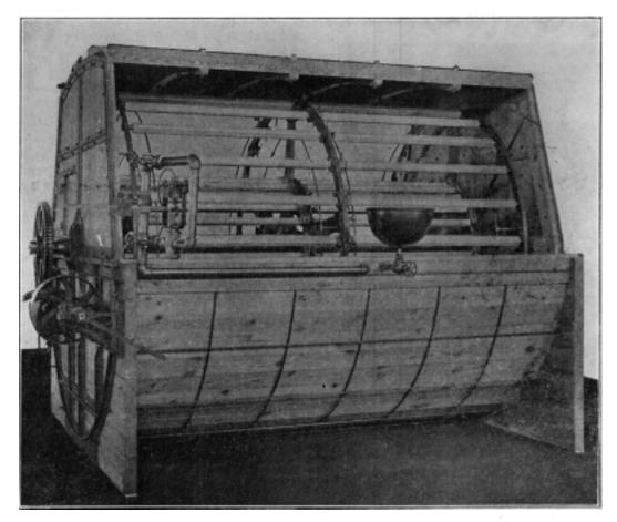
FIG. 1. THE GILES AUTOMATIC DYEING MACHINE FOR SKEIN YARN
