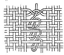
FIG. 2. SHOWING THE LAY OF THE BINDER THREAD
