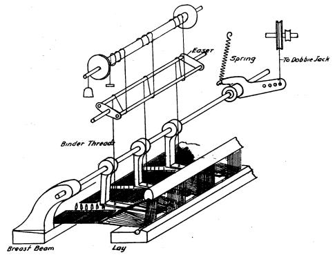
FIG. 5. THE DEVICE FOR WEAVING FILLING LENO
