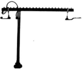
FIG. 3. THE INDUCTOR TILTED BACK FOR STRIPPING AND GRINDING
