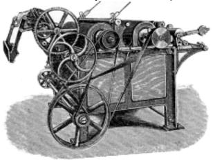
FIG. 2 A DOUBLE RAISING MACHINE WHICH IS ADAPTED FOR PIECE GOODS
