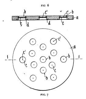
sists of a support, a, Fig. 6, which is not affected by acids. The metallic plates of gold or platinum are inserted at b. These plates are pierced with a capillary hole, c', and are fixed firmly in the supports. The support, a, Figs. 6 and 7, correspond to 6, Figs. 1 and 2, the illustrations showing clearly the method of construction.
