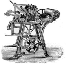
FIG. 3. A SINGLE RAISING MACHINE FOR PIECE GOODS
