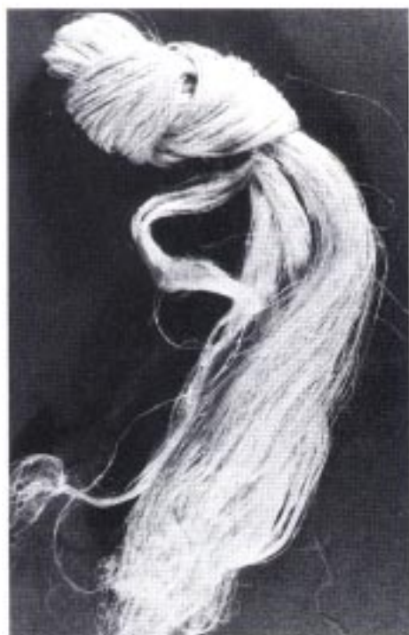
4. Pineapple fiber. The longer fibers in the bundle measure 52”.
