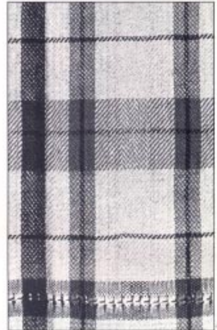
Above, alternate rows of twills and basket weave. Right, straight twill treading on straight twill and broken twill threading; one row of leno lace picked in. Four ends in the rose stripes were replaced with dark brown to weave an overcheck in the last towel on the warp.
