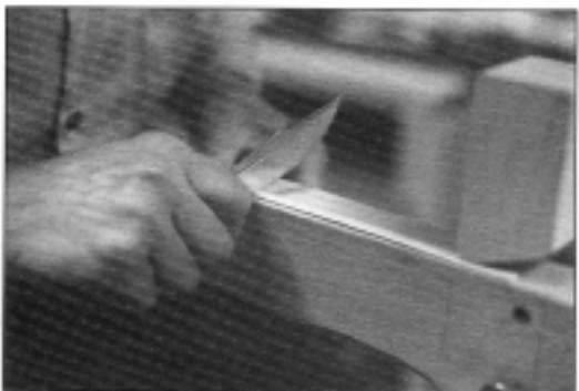
The dents were further refined and smoothed with a knife. Notches were cut in both ends to accommodate being installed in the reed spines.
