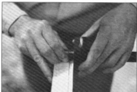
A marking gauge was used to lay out the prepared blank for slitting into individual dents.
