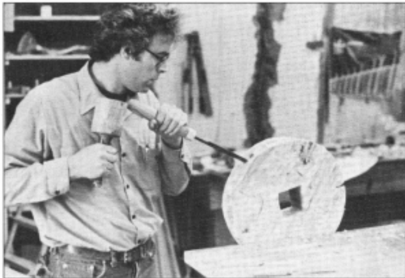
The front ratchet was made from two adzed cottonwood pieces, pegged together to resist splitting. Pockets were chiseled in the periphery of the wheel, and a stick was used to hold the ratchet.
