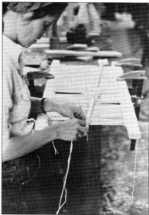
Left, harnesses fabricated from a bar on the top and a bar on the bottom and string heddles are not unlike those of present day Swedish looms.
