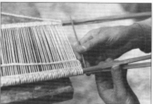
The spines for the reed were made from bamboo that was split and scraped smooth. Cotton string was plied until a thickness was achieved that gave the proper reed spacing. After the dents were inserted they were secured with a half hitch.
