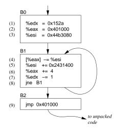
Figure 1. Structure of the unpacker routine for the Hybris-C email worm.
