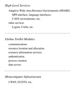
Figure 12.9 The components and structure of the Globus toolkit.
