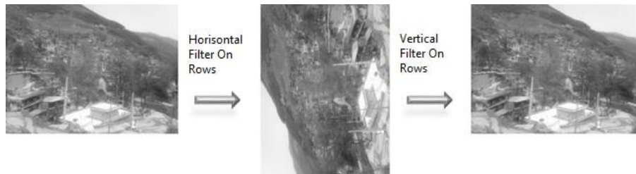
Figure. 2. To construct a GSS image, we first apply Gaussian filter on rows of pervious scale (Left image) while storing it in a transpose manner (Middle image), then apply same filter on rows to obtain next GSS image (Right image).
