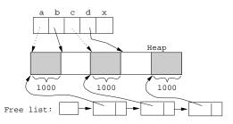
• Without compaction the last allocation will fail, even though enough memory is available.
