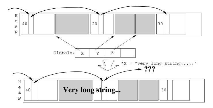
For this reason it's a good idea to have a magic number in the free list node headers. This is a distinctive value that malloc checks when traversing the free list, and complains if the value changes (which indicates the list is corrupted). For example, put a field in the header whose value is always 0xfeedface.
