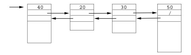
malloc should return a word-aligned region that can store integers. The easiest way to do this is to start with the heap word-aligned, and always allocate memory in multiples of the word size.
